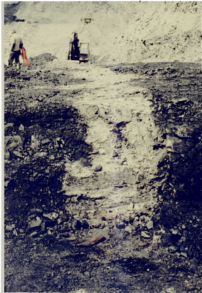
Plate 2.3 : A : Abandoned workings showing haulage roadway totally infilled by seat earth clay which has 'squeezed' or 'puffed' from beneath the coal seam (South Staffordshire Coalfield).
