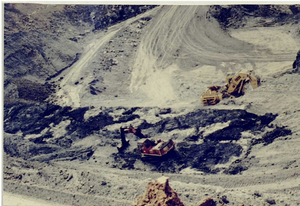
Plate 2.3 : B : Areal view from opencast site highwall showing the complex of coal workings infilled by seat earth clay (South Staffordshire Coalfield).
